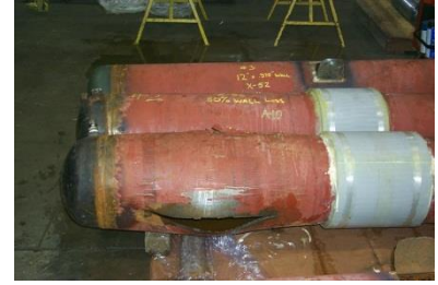
Pipe Body Failure @ 4,260 psi
